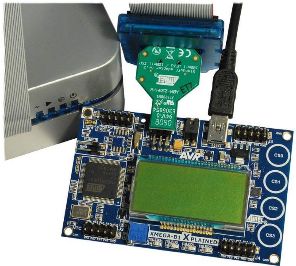
Figure 4-3. Connecting the Atmel AVR ONE! debugger to the Atmel AVR XMEGA-B1 Xplained board.
