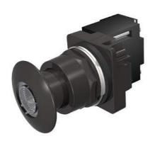
30mm BlackMax, Epoxy Coated Corrosion Resistant Complete Metal Unit Illuminated Push-Pull Operator Transformer type, 120V AC LED Lamp Mushroom Head Cap Small 1 3/4" (44.5 mm) Metal, Black with Clear Lens 2 Position Maintained, Pull-to-Release UL Listed, CSA Certified NEMA 1,3,3R,4,4X,12,13 & Automotive Standards
