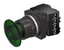
30mm BlackMax, Epoxy Coated Corrosion Resistant Complete Metal Unit Illuminated Twist-to-Release Full Voltage, 24V AC/DC LED Lamp Mushroom Head Cap Small 1.79" (45 mm) Plastic Cap, Green 2 Position Maintained, Twist-to-Release with 1 N.O. - 1 N.C. Heavy Duty Contacts, A600/P600 UL Listed, CSA Certified NEMA 1,3,3R,4,4X,12,13 & Automotive Standards
