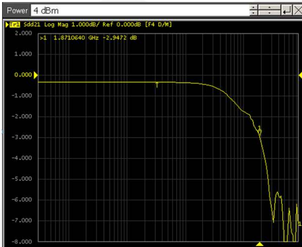
Figure 17. MHL Path SDD21 Insertion Loss Curve
