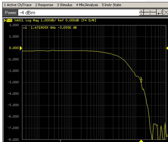
Figure 18. USB Path SDD21 Insertion Loss Curve
