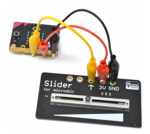
Its a good idea to use the red lead for 3V, black for GND and a different color to connect the output of the Slider for micro:bit to your BBC micro:bit. You can use P0, P1 or P2 of your micro:bit, but for the example programs here, it is assumed that you have connected it to P2 as shown above.
