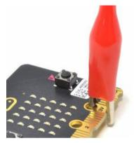
Connecting the alligator clips like this prevents any accidental connections between the large connectors with the holes in and the much smaller connectors (gold lines in the photo above)
