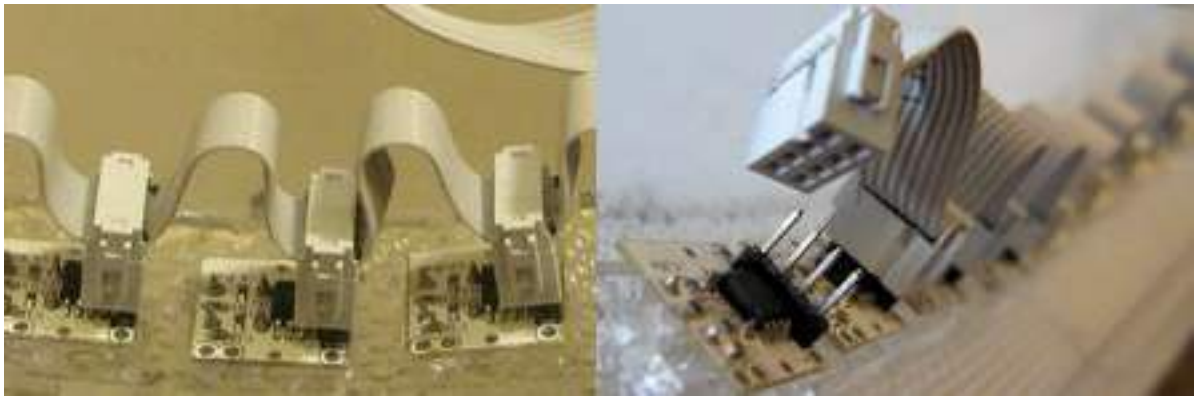
Photo 4.2: BlinkM I2C bus with IDC connectors and ribbon cable
