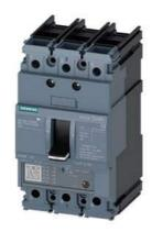
circuit breaker 3VA5 UL frame 125 3-pole, starter protection TM120M, AM, In=80A without overload protection short-circuit protection li=3...7 x In nut keeper kit on both sides
