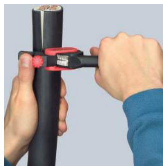
Turning the tool for circumferential cut
