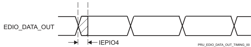
Figure 7-111. PRUSS IEP Digital IOs Timing Requirements
