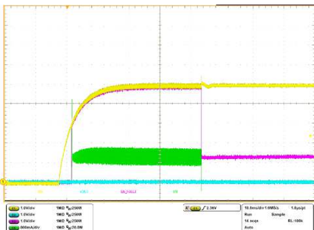
Figure 26. Startup into output short-circuit
