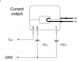
S25P100D15Y At  $I_f$  = 100A &  $V_{CC}$  = ±15 $V_{DC}$ 20Ω ≤  $R_M$  ≤ 102Ω
