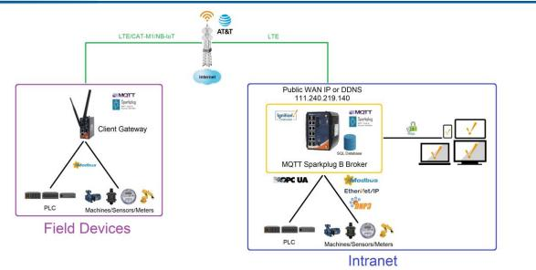
Ignition MQTT Broker installed onboard in IGMG-P83244GC+-D4G Gateway makes the system self-contained and more cost effective when a Cloud server does not have to be used. End-devices can access the MQTT server remotely and directly with its Public WAN IP or DDNS address. Ignition running in user's premises can work with local clients and devices and simultaneously provide a possibility of data visualization and storage as well as end-devices control via cellular link.
