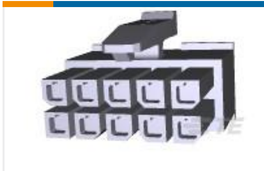
TE Part #1-794617-0 10POS,MICRO MNL,RCPT HSG
