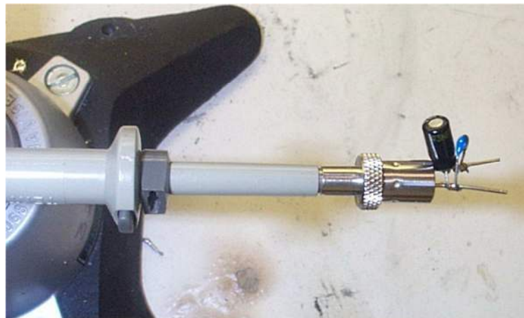
Figure 47 – Oscilloscope Probe with Probe Master ( www.probemaster.com ) 4987A BNC Adapter. (Modified with wires for ripple measurement, and two parallel decoupling capacitors added)
