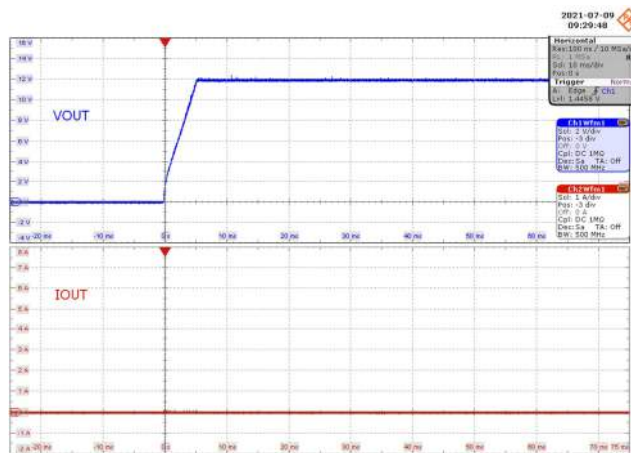
Figure 22 – Output Voltage Start-up. 90 VAC, 0% Load. Ch1/Upper: V_{OUT} , 2 V / div. Ch2/Lower: I_{OUT} , 1 A / div. Timebase: 10 ms / div.
