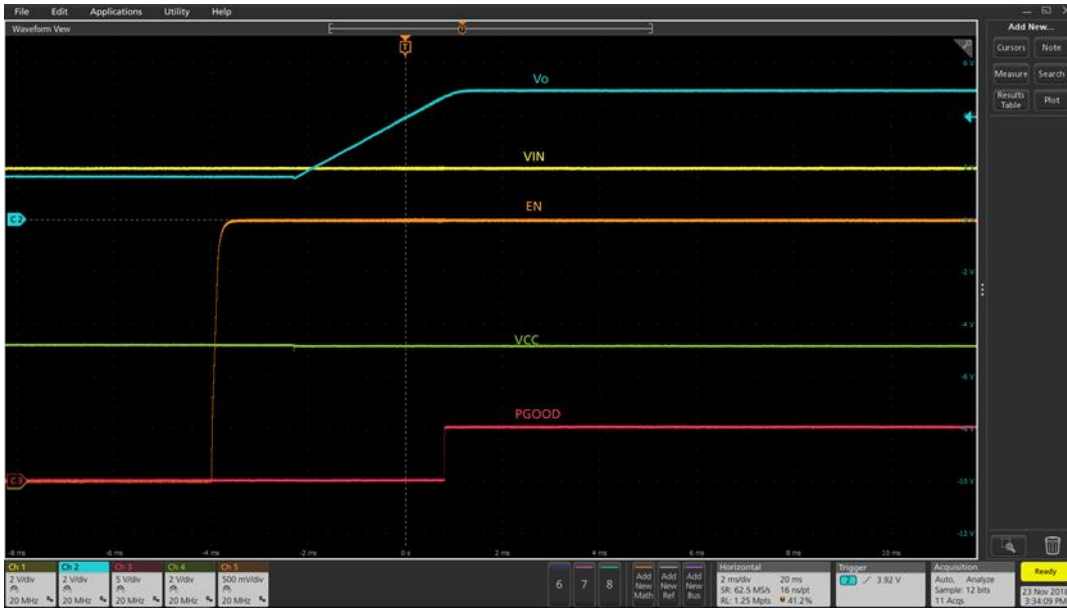
Figure 20 Startup into pre-bias (Ch1:PV IN , Ch2: V OUT , Ch3: PGood, Ch4:V CC , Ch5: Enable)
