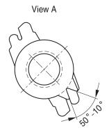
Hole arrangement View in mounting direction
