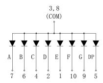
Internal Circuit Diagram (Common Cathode)
