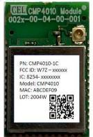
Surface-mount PCB Trace Antenna Antenna Connector Castellation Edge 16.7 x 26.3mm
