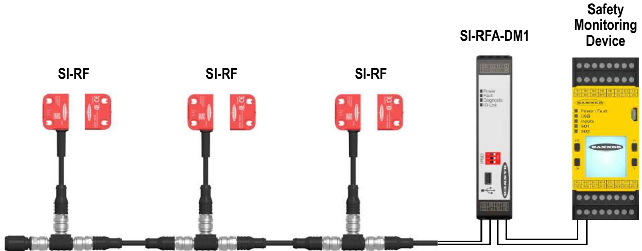
Figure 3. Connecting the SI-RF in series with a DM1 and monitoring device
