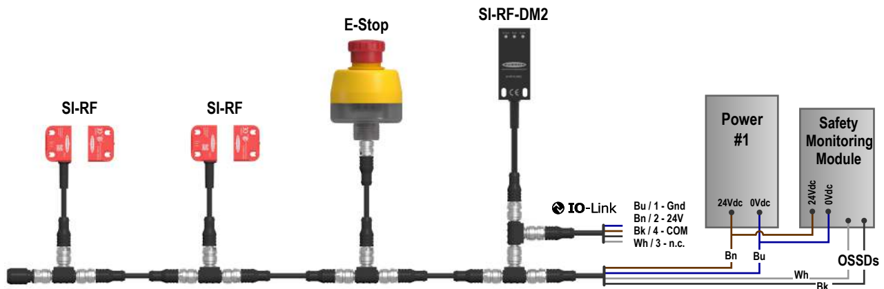
Figure 4. The SI-RFA-DM2 can be connected using a t-adaptor (SI-RFA-TS) connected to a reset t-adaptor (SI-RFA-TK)
