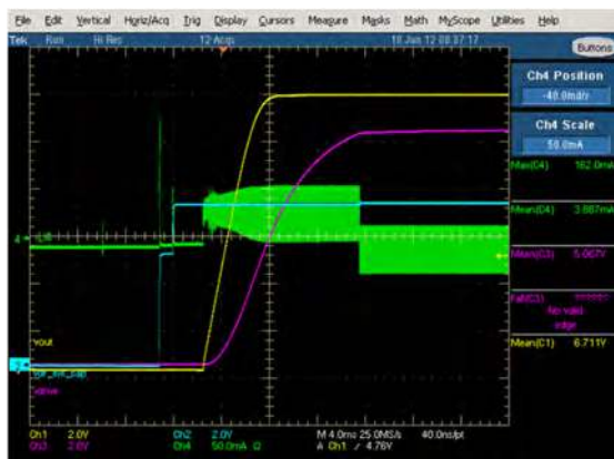
Figure 5. Soft-Start with Vout connected to Vdr_ext with diode +20 Ω 200μF Yellow=Vout, Purple=Vdr_ext Blue=Vdr, Green=IC current
