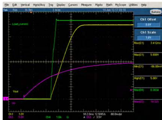
Figure 3. Start-up 15Vin Vo=5.8V, 6A, 5MHz
