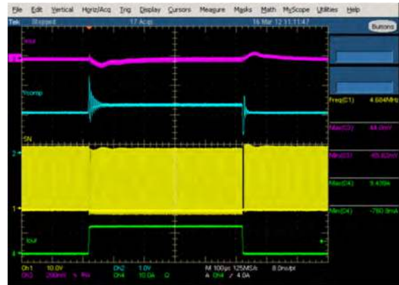
Figure 40. Transient step response Vin=24V, Vo=5V 5MHz 1-7A, Fc=600kHz Ch1 (yellow): Switching node, Ch2 (blue): COMP, Ch3 (purple): Vo, CH4 (green): Io
