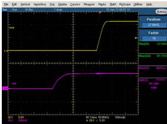
Figure 1. Vref and Vout start-Up Vin=48V Vo=12V
