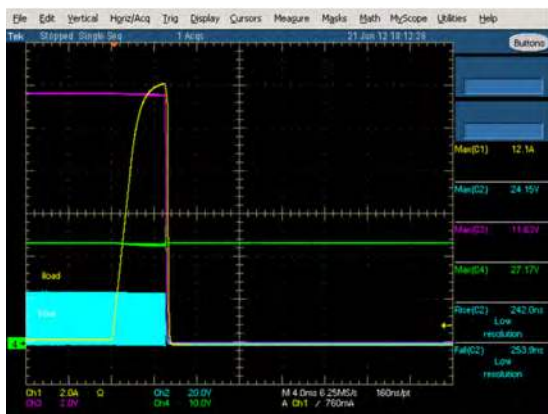
Figure 17. Current limit operation Rds_on= 13mΩ, Rlim=128kΩ Ch1 (yellow): output current, Ch2 (blue): switching node Ch3 (purple): output voltage, Ch4 (green): input voltage
