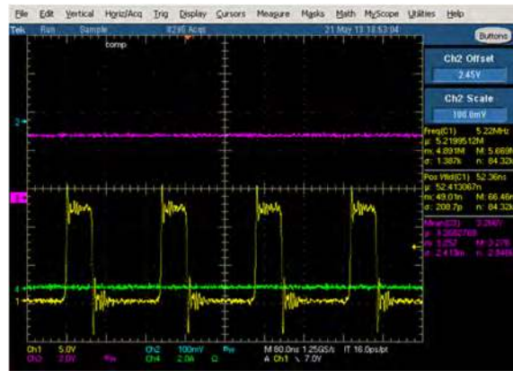
Figure 41. Steady state operation Vin=12, Vo=3.3V 5MHz No load Ch1 (yellow): Switching node, Ch3 (purple): Vout, CH4 (green): Io
