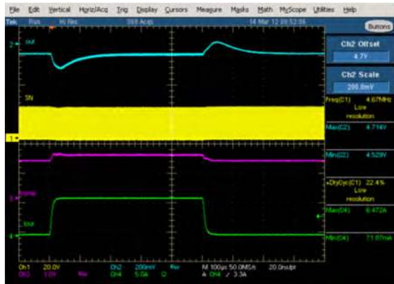
Figure 39. Transient step response Vin=24V, Vo=5V 5MHz 1-7A, Fc=140kHz Ch1 (yellow): Switching node, Ch2 (blue): Vo, Ch3 (purple): COMP, CH4 (green): Io
