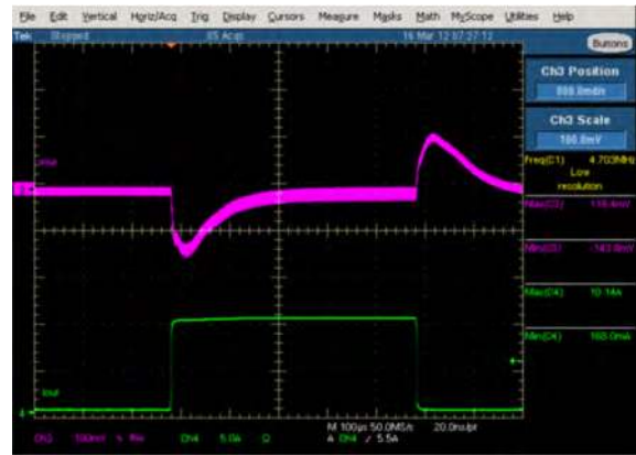
Figure 38. Transient step response Vin=24V, Vo=5V 5MHz 1-10A Fc=140kHz
