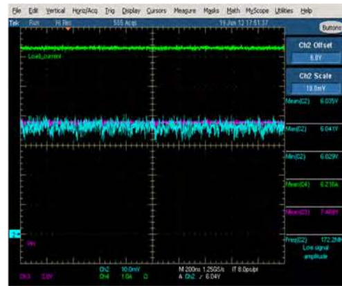
Figure 32. Ripple 8Vin Vo=6V, 6A 5MHz
