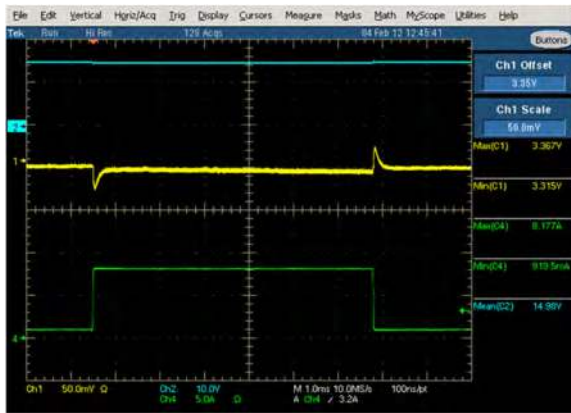
Figure 37. Transient step response Vin=15V, Vo=3.3V 2.2MHz 1-8A
