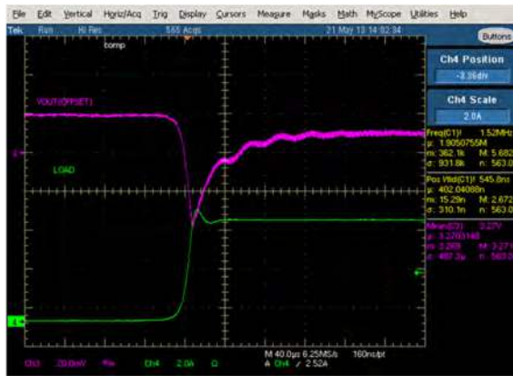
Figure 43. 0-5A step load V_{in}=12 V_o=3.3V f_{sw}=5MHz , Ch3 (purple): V_{out} , CH4(green): I_o
