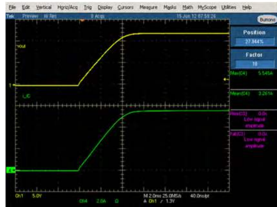
Figure 2. SS Vin=24V, Cref=1nF, CVdr=1μF, Cv3V=1μF, css=68nF, Io=5.5A
