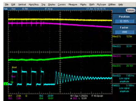
Figure 18. Expanded Current limit operation Rds_on= 13mΩ, Rlim=128kΩ Ch1 (yellow): output current, Ch2 (blue): switching node Ch3 (purple): output voltage, Ch4 (green): input voltage.
