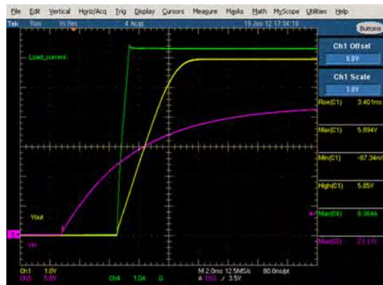
Figure 4. Start-up 22Vin Vo=5.8V, 6A, 5MHz
