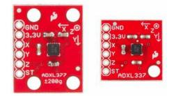
As you can see, each breakout has the same pins broken out. Here is some information about each pin:
