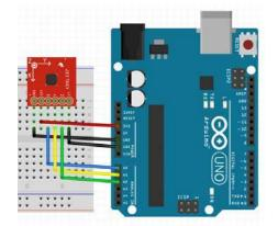
We simply have to supply the accelerometer with power (3.3V and GND), then hookup the X, Y, and Z lines of the sensor to ADC pins (A0, A1, and A2 respectively in this case). The self test pin (ST) can be left disconnected or connected to ground under normal operation. If you want to use the self test to double check the functionality of the sensor, tie it to 3.3V. Check the datasheet for more info.
