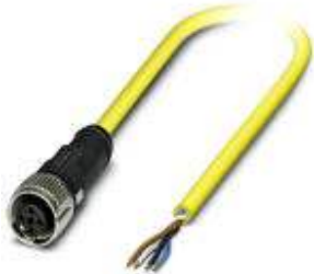
Sensor/Actuator cable, 4-position, TPE, yellow RAL 1021, free cable end, on Socket straight M12 SPEEDCON, A-coded, Cable length: 10 m
