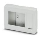
Display housing, 5.7", light gray, consisting of two half shells with screws, window on the left. Front 1.1 mm recessed, keypad area on the right recessed for wall installation
