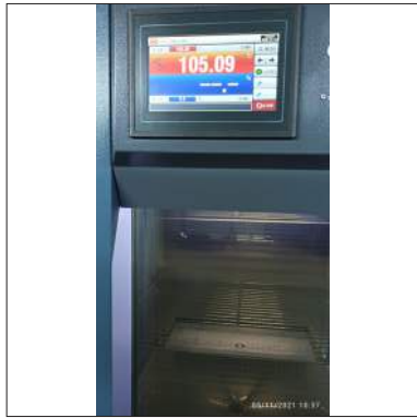
Temperature stress in the climatic chamber
