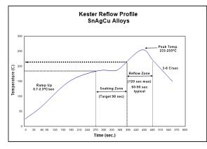
The recommended reflow profile for formula made with SAC and SnAg alloys is shown here. This profile is simply a guideline. WP616 has excellent solderability and wetting across a wide range of profiles, with similar performance in air and nitrogen. Your optimal profile may be different from the one shown based on your oven, board and mix of defects. Contact Kester Technical Support if you need additional profiling advice.
