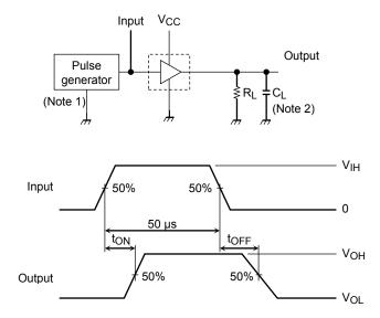
Note 1: Pulse width 50  $\mu$ s, Duty cycle 10% Output impedance 50  $\Omega$ ,  $t_{\Gamma} \le 5$  ns,  $t_{f} \le 10$  ns,  $V_{IH} = 5.0$  V
