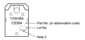
Note 2: A line under a Lot No. identifies the indication of product Labels. Not underlined: [[Pb]]/INCLUDES > MCV Underlined: [[G]]/RoHS COMPATIBLE or [[G]]/RoHS [[Pb]]
