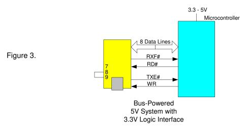
Figure 3 shows how to configure the DLP-USB1232H to interface with a microcontroller via the parallel 245 FIFO interface mode. In this example, the target electronics can operate at from 3.3 - 5 volts since the DLP-USB1232H interface I/O pins are 5 volt tolerant.
