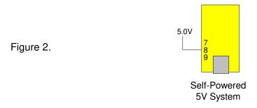
Figure 2 illustrates a typical USB self-powered configuration. A USB self-powered device gets its power from its own power supply and does not draw current from the USB bus.
