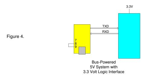
Figure 4 shows how to configure the DLP-USB1232H to interface with a 3.3V logic device via the ASYNC serial mode. In this example, the target electronics provide the 3.3 volts to power the microcontroller.
