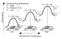
The temperature of the resistor will increase the same riangle T from the standard terminal part temperature regardlless of the ambient temperature when the same power is applied. This is because there is hardly any heat dissipation from the resistor surface to the ambient air.
