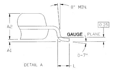
DIMENSIONS ARE IN MILLIMETERS
