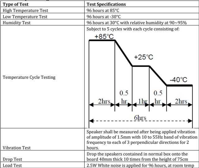
After each test let rest for 6 hour at 25°C, then the part shall be within ±3 dB.
