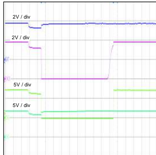
Figure 14. Undervoltage Protection Set and Clear
