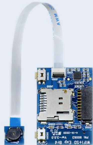
Add-On Board with optional Chirp Ultrasonic Time-of-Flight Sensor
