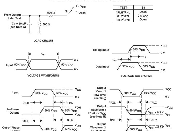
NOTES: A. C<sub>I</sub> includes probe and jig capacitance.
