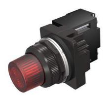
30mm BlackMax, Epoxy Coated Corrosion Resistant Complete Metal Unit Illuminated Indicator Light Full Voltage type, 6V AC/DC Super Bright LED Lamp, BA9s Glass Lens, Red UL Listed, CSA Certified NEMA 1,3,3R,4,4X,12,13 & Automotive Standards
