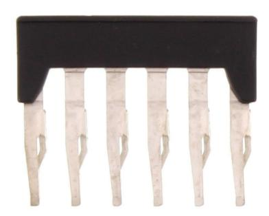
Insulated cross-connector, No. of poles: 6, Mounting type: Plug in, Width: 29.5 mm, Rated cross-section: 2.5 mm², Colour: Black
