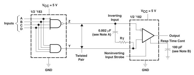
NOTES: A. When the inputs are open circuited, the output is high. A capacitor may be used for dc isolation of the line-terminating resistor.
