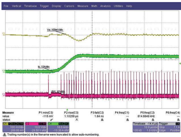
Fig. 29 - Load Step, 0.1 A to 12 A, 1 A/ \mu\text{s} , t = 10\ \mu\text{s}/\text{div} Skip Mode Enabled
