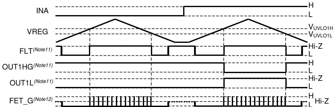
Figure 76. VREG UVLO Function Operation Timing Chart
