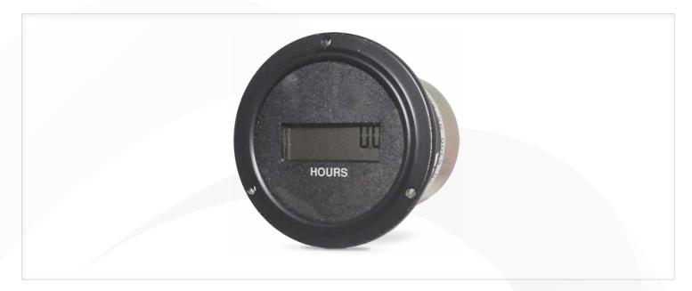
The Model 720 Electronic Hour Meter offers a large 8 digit LCD display, (99999999.9) 0.32" (8mm) high, with an input operating voltage of 85-500VAC. The front of the unit is totally sealed, and the Hour Meter is housed in a rugged steel enclosure that is interchangeable with the Redington Model 720 Electro Mechanical Hour Meters. The wide operating voltage makes this product ideal for almost any application.
