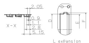
Emboss taping specification (Based on taping of electronic parts [JIS 0806])
