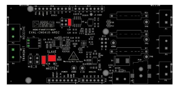
A transformer or a pair of transformers are used to isolate the signals between the two LTC6820's and must be terminated by a resistor. Only the master and the last slave on the transmission line must be terminated by shorting connectors P5 and P7
