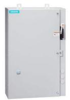
Non-reversing motor starter Size 4 Three phase full voltage Solid-state overload relay OLRelay amp range 50-200A 220-240/440-480VAC 60HZ coil Combination type 150A circuit breaker Enclosure NEMA type 4/12 Water/dust tight for outdoors Standard width enclosure
