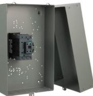
Electrically held lighting contactor, Contactor amp rating 100A, 0 N.C. / 3 N.O. Poles, 24VAC 50/60HZ coil, 1 NO / 1 NC auxiliary contacts Non-combination type, (no disconnect device), Enclosure NEMA type 1, Indoor general purpose use
