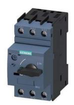
Special type Circuit breaker size S00 for motor protection, Class 10 A-release 0.9-1.25 A N-release 16 A screw terminal Standard switching capacity Ambient temperature -50  $^{\circ}$ C 500 switching cycles
