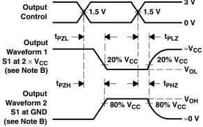
**VOLTAGE WAVEFORMS OUTPUT ENABLE AND DISABLE TIMES**
