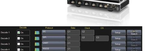
Simultaneously decode up to 4 serial data buses. When using the MSO option on WaveRunner Xi or WaveSurfer Xs the digital inputs D0, D1, D2, etc. can be used as the source for a serial data trigger and decode.
