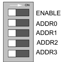
Figure 1-9: Configuration DIP Switch (SW13)
