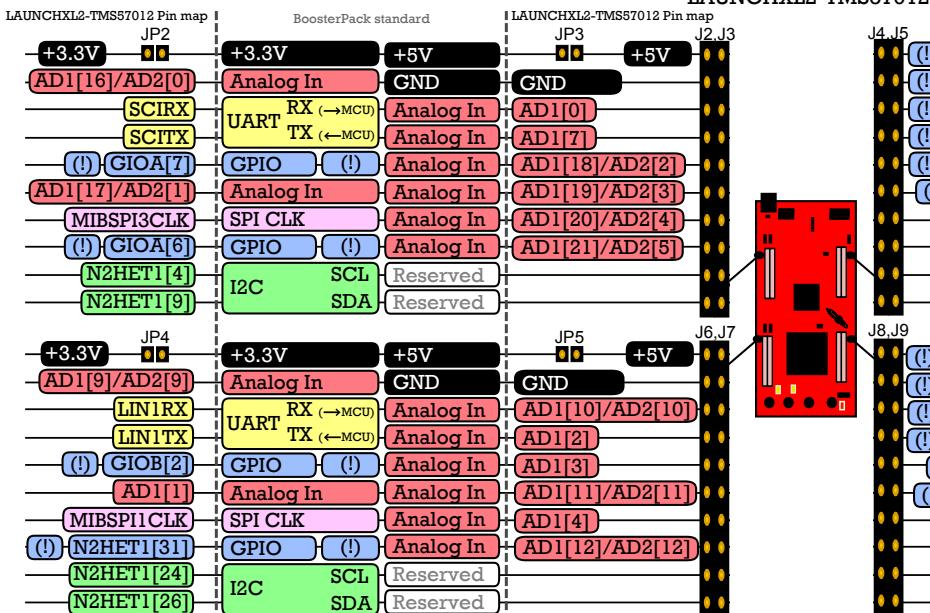
When using some BoosterPacks, JP2, 3,4, or 5 may need to be removed. For example, using this LaunchPad with BoosterPack BOOSTXL-DRV8301 that includes a 3.3V regulator. To avoid conflict between the LaunchPad's 3.3V regulator and the regulator on the BoosterPack, JP2 (or JP4) should be removed.
