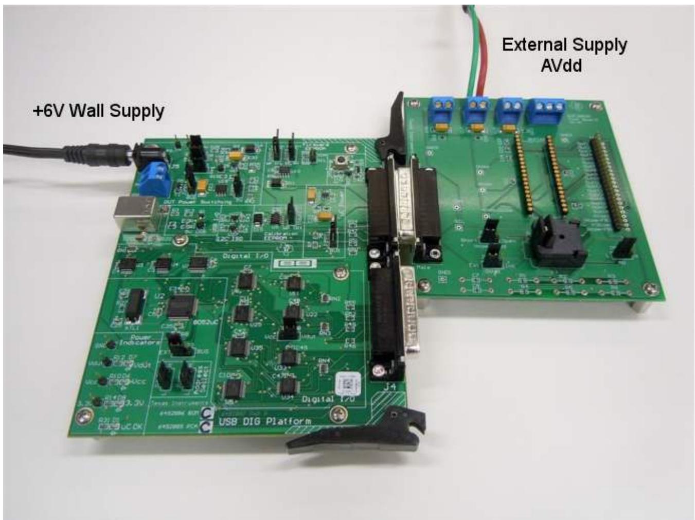
Figure 6. Connecting External Power to the EVM
